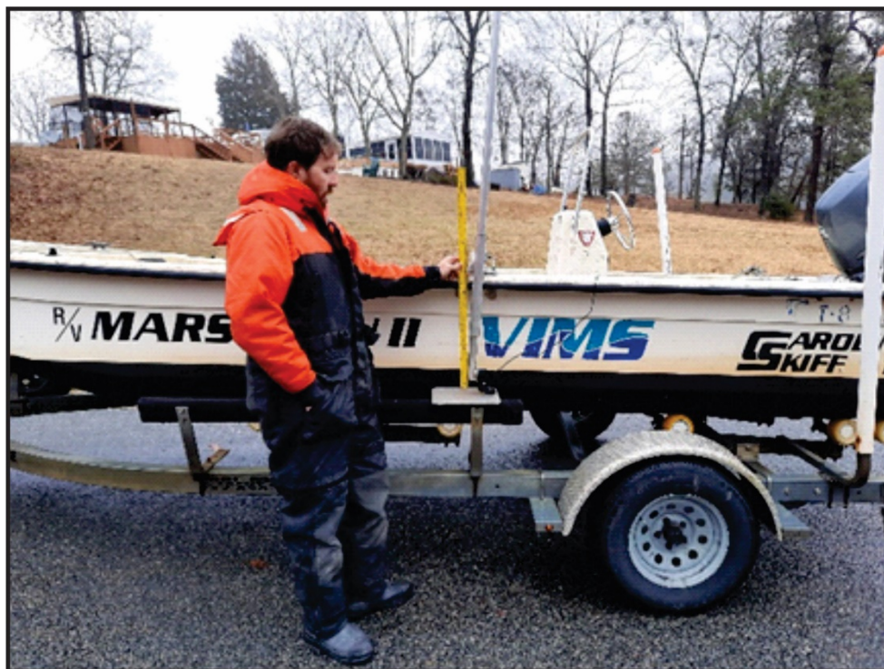
Figure 5. 19 ft Carolina Skiff with transducer attached to side.
