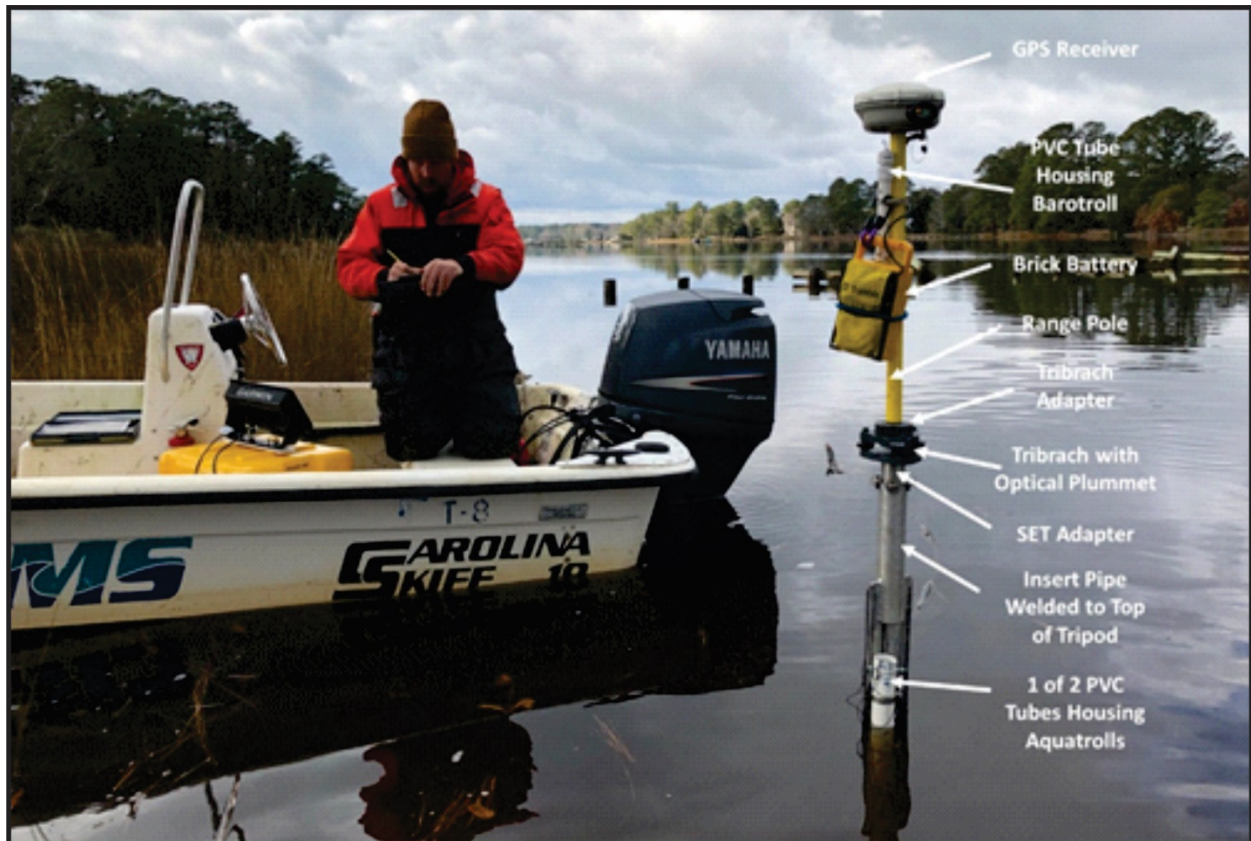
Figure 4. Water Level Tripod with attached GPS Receiver
