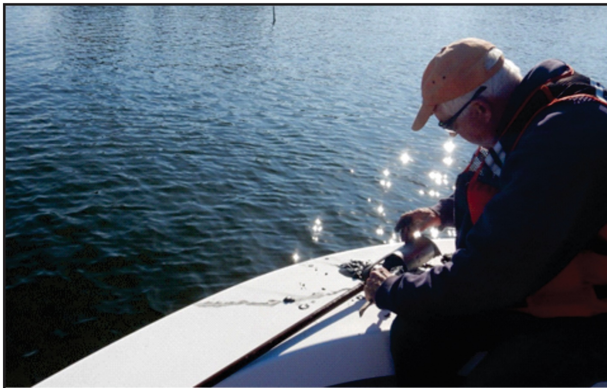
Figure 7. Sediment being removed from auger. Photo taken at Mill Creek in Middlesex County, VA.
